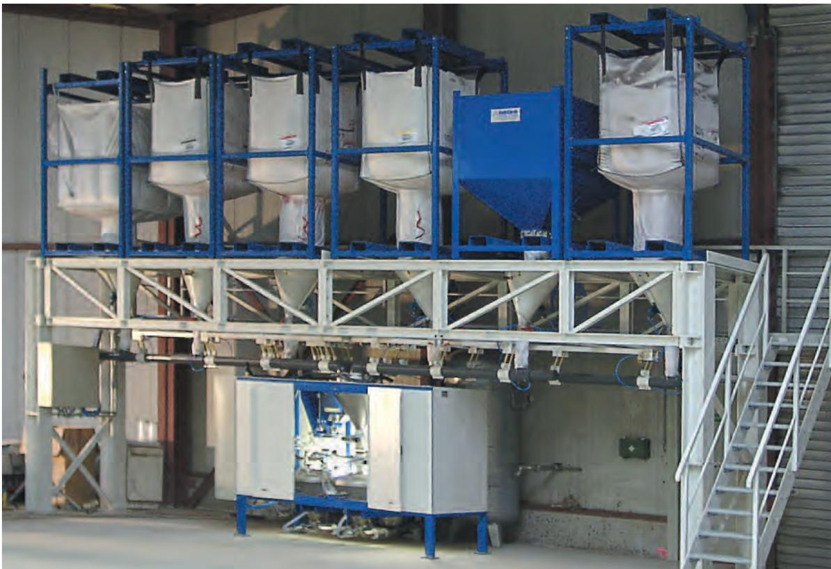
▲ **COM 70-3** Granular metering system with three conveying vessels for 6 colors in 3 mixers with one electronic weigh hopper
