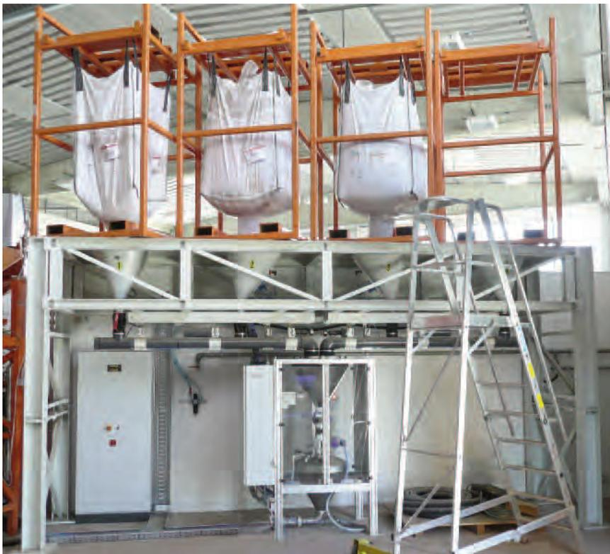
▲ **COM 70-1** Granular metering system with one electronic weigh hopper and one conveying vessel for 4 colors in 2 mixers with diverter valve
